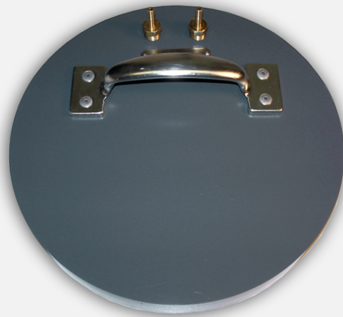
Surface Emission Chamber
