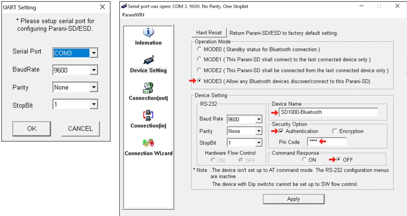
**Figure 2: ParaniWin UART Setting Dialog (Left) and Device Setting Panel (Right).** These windows are used to locate the SD1000 adaptor and configure the adaptor, respectively. Controls marked with red arrows must be modified from their factory defaults in order for the SD1000 to function properly with the RAD7.
