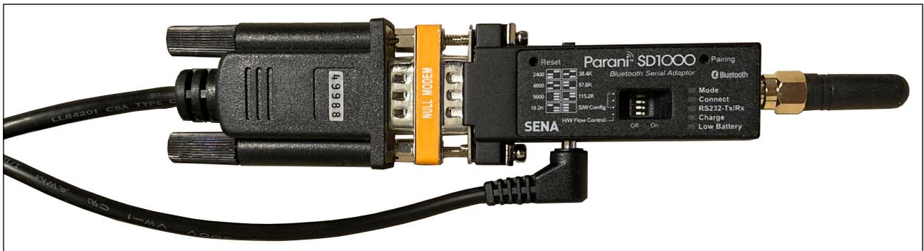
**Figure 1: Connecting the SD1000 to the computer.** This requires the Null Modem adaptor and a StarTech serial to USB adaptor cable.
