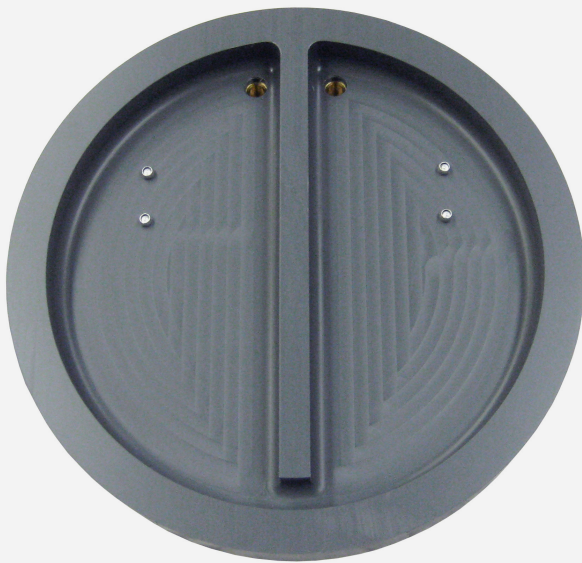
Figure 6 Hard Surface Emission Chamber (Left)
