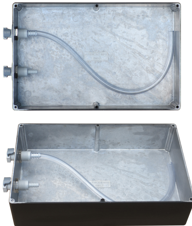
Figure 5 Bulk Emission Chamber uncovered (two angles)
