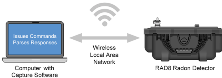
Figure 1: Using Capture software to connect to a RAD8 over a wireless local area network.
