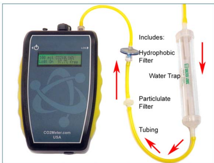
Figure 6: Filter Installation and Orientation
