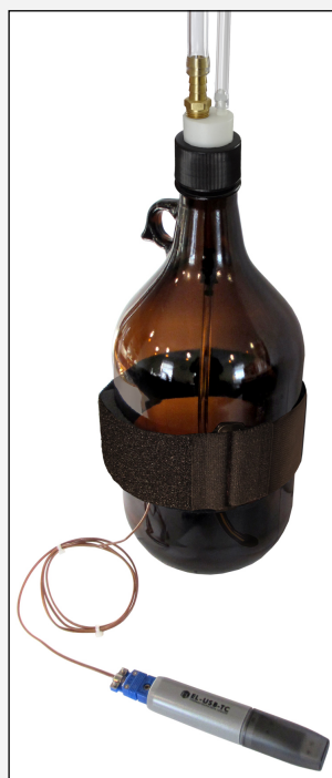
Figure 4 Aerator and Bottle assembly with Temperature Logger
