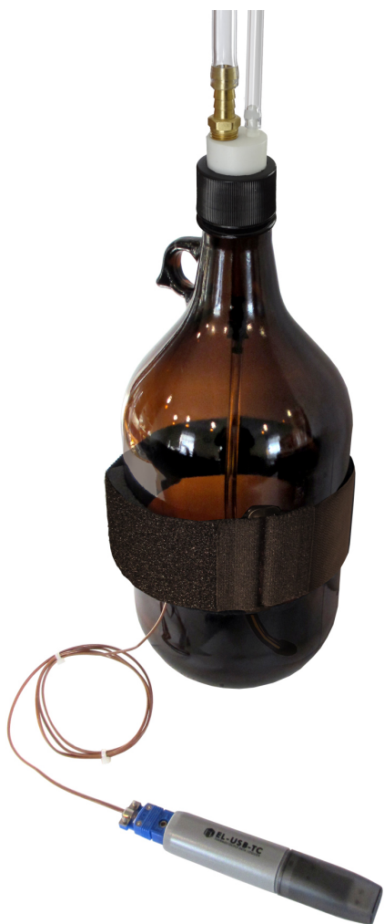
Fig. 4 Aerator and Bottle assembly with Temperature Logger
