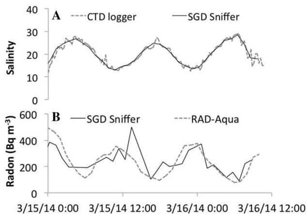
**Fig. 3** **a** Salinity in coastal surface water measured by a salinity probe (dashed line) and calculated based on the <sup>40</sup>K activity determined by the SGD Sniffer (solid line). **b** Radon in coastal surface water measured via the RAD-Aqua radon in-air monitor (dashed line) and through <sup>214</sup>Bi using the SGD Sniffer (solid line)
