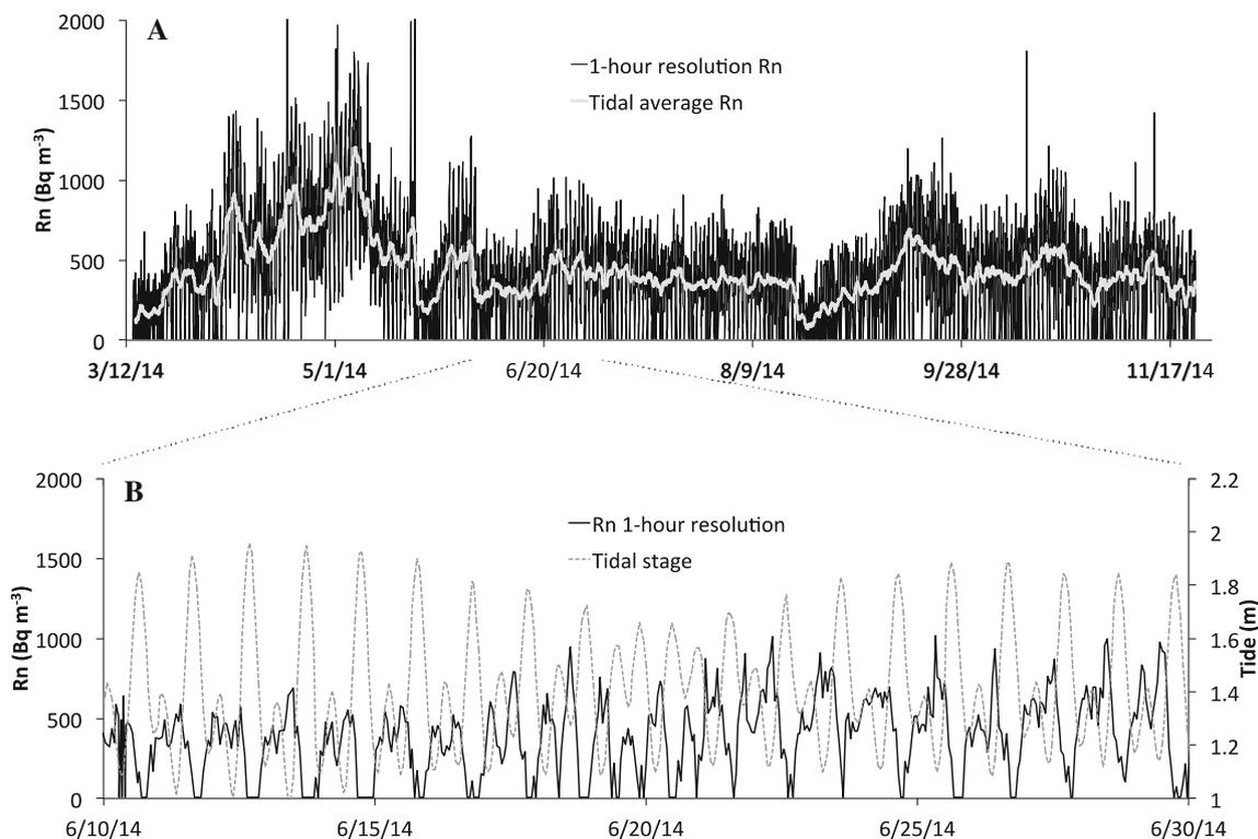
**Fig. 2** **a** Radon activities recorded by the SGD Sniffer in Kiholo Bay, HI at hourly resolution (black line) and running averages over a tidal cycle (gray line). **b** Radon was negatively correlated with tidal stage (gray dotted line) throughout the deployment
